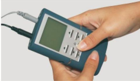
In order to turn on the device, keep the [
